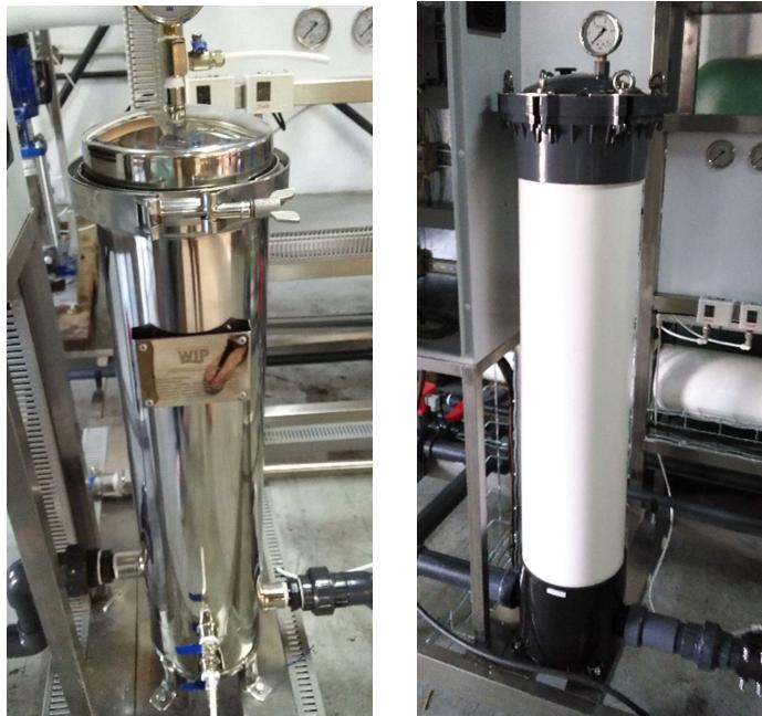
Multi-cartridge filter image in stainless steel and PVC respectively.
